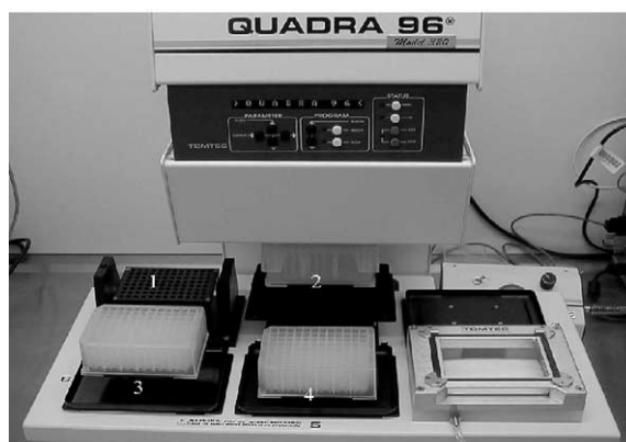
1. Tip Reservoir 2. Acetonitrile Reservoir 3. Supernatant Destination Plate (1-mL/well) 4. Original Sample Plate (2-mL/well)
